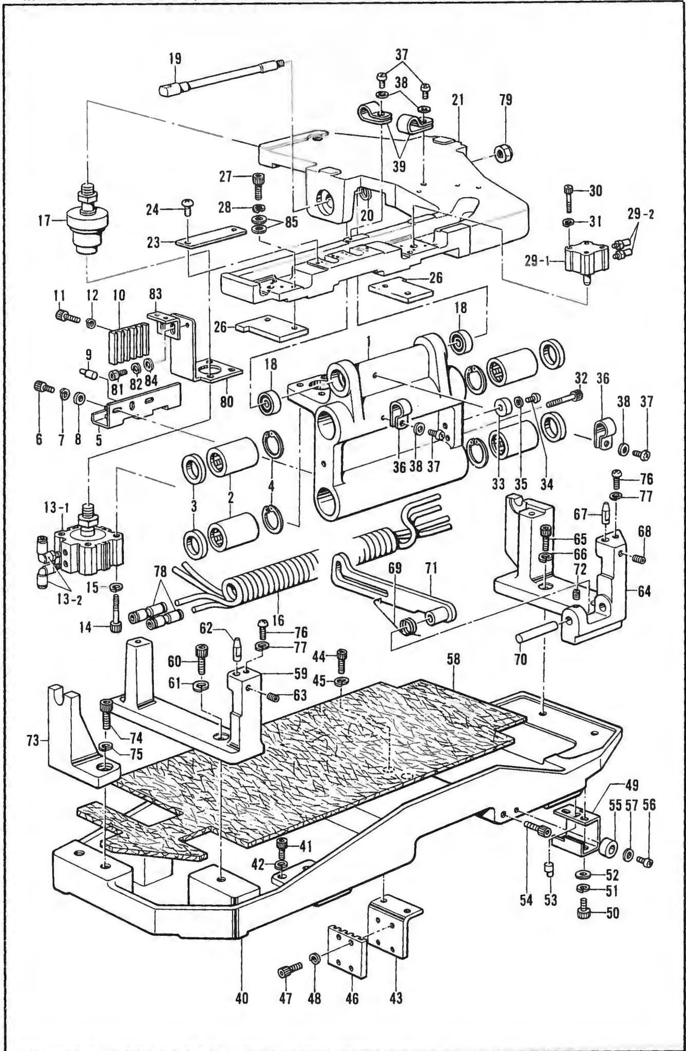
H. 駆動側・送り関係/Drive, feed mechanism/Transportvorrichtung/
