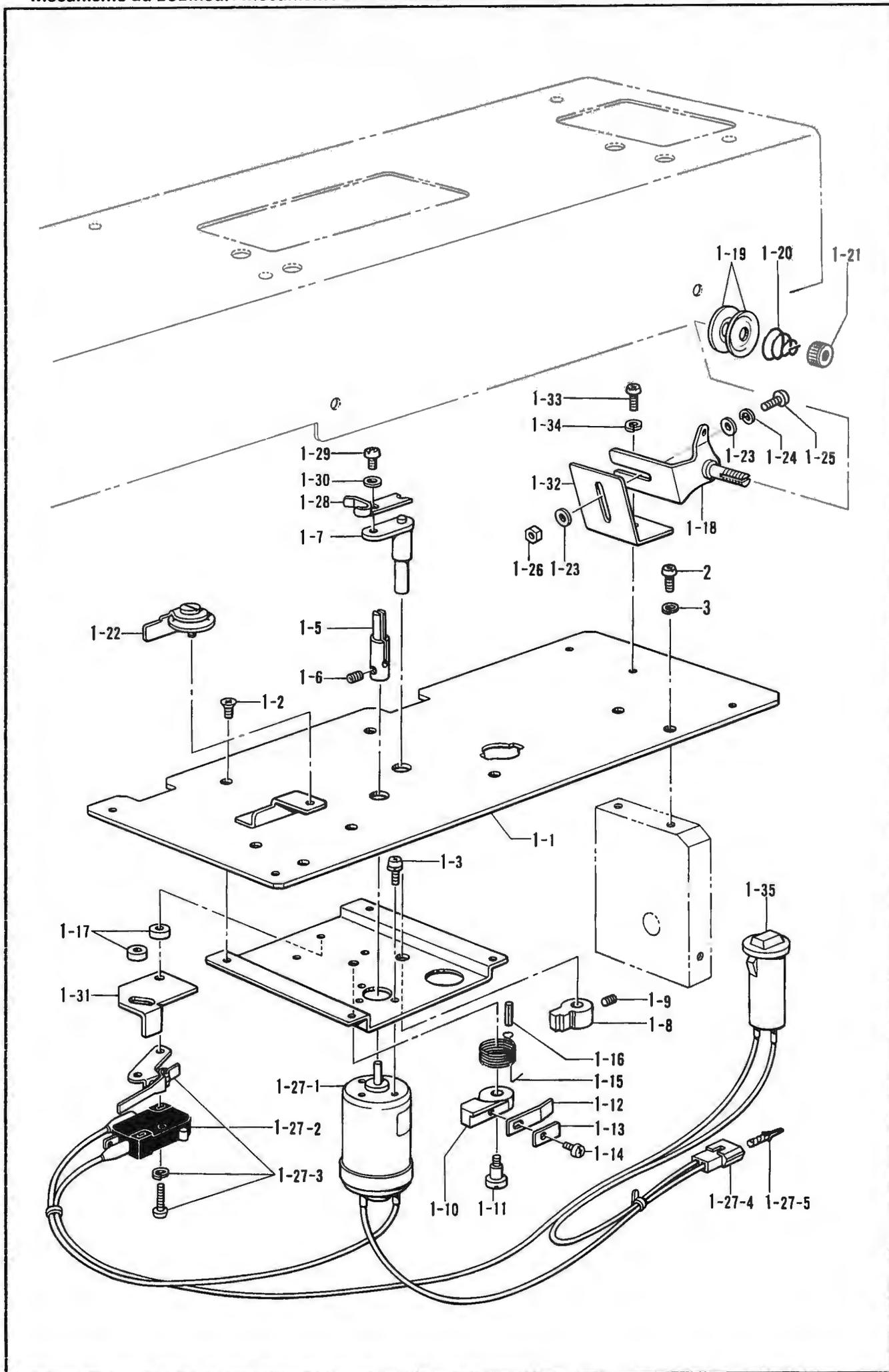
Q. 糸巻関係 / Bobbin winder mechanism / Spuler /
